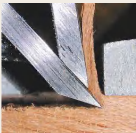
▲ Pic.5 Planing against the grain, using a cap iron and a fine shaving aperture
